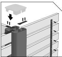
Lock in top slat with bracket and 2 screws. Mark and drill holes in the brace strip to line up with the back of each slat. Fix in place with 15mm button-head screws. Replace cap.
