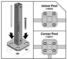
Mark & drill the four anchor holes, noting fastener positions shown above.
